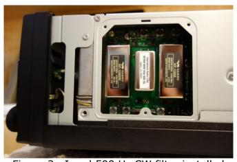
Figure 2. Inrad 500 Hz CW filter installed
