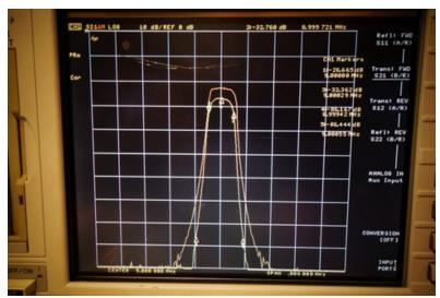
Inrad 500 Hz filter vs. Stock 600 Hz filter
